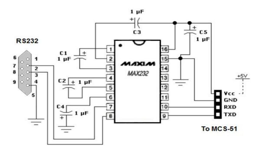
13)Draw hardware block diagram and write software assembly program code (without ISR) to design digital circuit for communicating between 2 computers through RS232 based on AT89C51. The first computer for sending data-bytes whiles the second computer for receiving them with baud rate 9600 (TH1=FDh).
