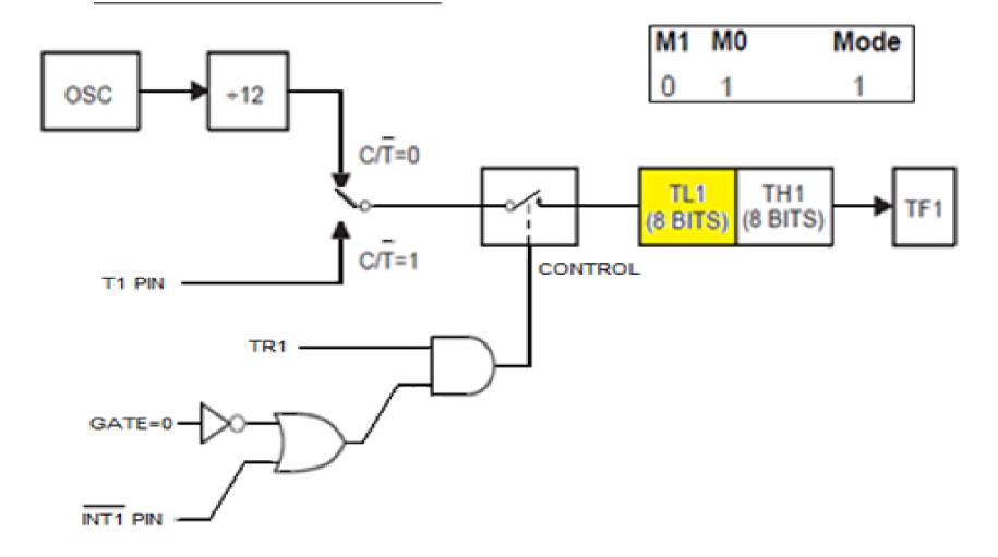
9) An embedded system is designed to count the instantaneous number of cars during enter a park. The system makes alarm and closes the door if it counts equal 400 cars. Write assembly code to perform the mentioned task (without using interrupt) based on Timer 1 of AT89C51.
