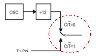
Gate .... For enable/disable the external interrupt to run/stop timer
